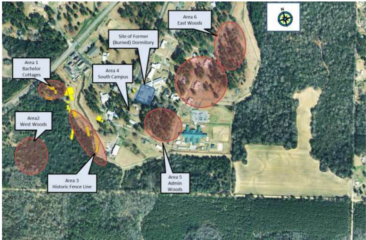
Figure 69. Illustration of additional search areas. Yellow squares are locations of GPR analysis. The red circles include areas of exploratory GPR surveys in which the data was not processed but in field assessments were made with probing, test pits, and mechanical trenching to look at soil profiles.
