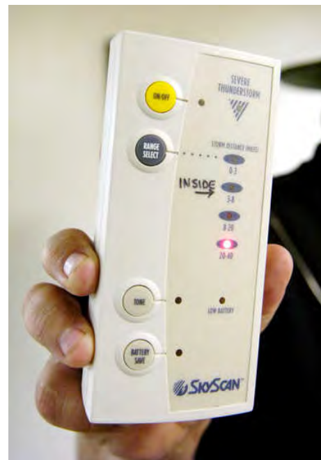
A similar lightning detector in use at a Bonaire GA football game had prompted officials to begin moving people off the field when lightning struck
