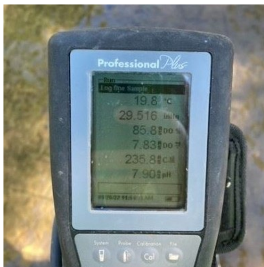
YSI Professional Pro multi parameter field meter
